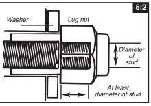
wheel spacer must not reduce the minimum permitted thread engagement below the limits established by fastener diameter. (See example as stated above.) No stacking of wheel spacers allowed. Maximum rim width on any car: 16 inches. No rear wheel discs or covers permitted in any category. Top Fuel and Funny Car rear wheels must meet SFI Spec 15.4. Pro Stock, Top Alcohol Dragster, Top Alcohol Funny Car, and Pro Modified (Comp) must meet a minimum of SFI Spec 15.1.
