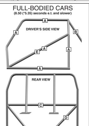
All cars with an OEM steel frame must have roll cage welded to frame. For 1997 and later Z06 and ZR1 Corvettes only with aluminum frames, the acceptable roll-cage mounting is shown in the next drawing.
